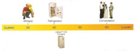
Carrier manufactures gas furnaces that are among the quietest in the industry. We test our products in a sound laboratory specifically built to semble a typical residence. Sound lavel recordings produced at steady state, low fire operation (the most common operating condition), measure 3 feet from furnace. Other sound levels, mentioned for compenion, as published at http://www.nidod.nih.gov/hearity/fiearing.ruler.asp.
